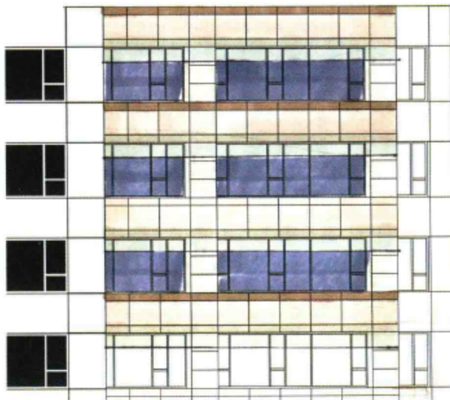
RESIDENTIAL TOWER FACADE: Fins and metal panel banding visually tie windows and skin system of the residential tower together. This simplifies the facade while giving it more character. This unifies facade and allows for interesting lighting and larger scale patterning to occur.
